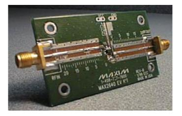
Objective: To tune the MAX2640 for operation at 345MHz for wireless security-system
